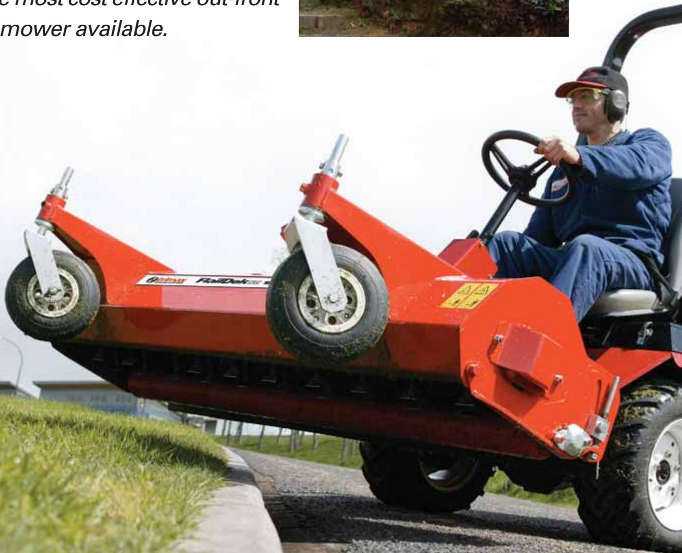
*Lifts high for climbing kerbs or loading onto trailers.*
